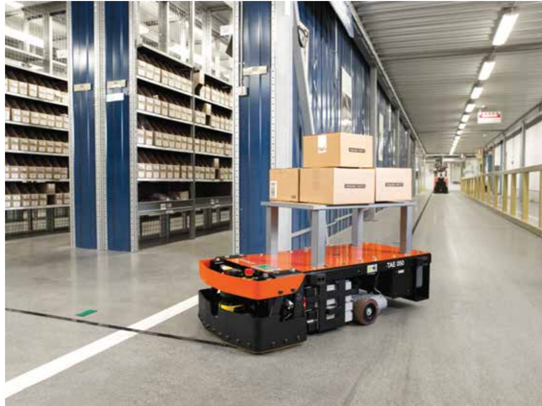
TAE050 carries load along magnetic tape
